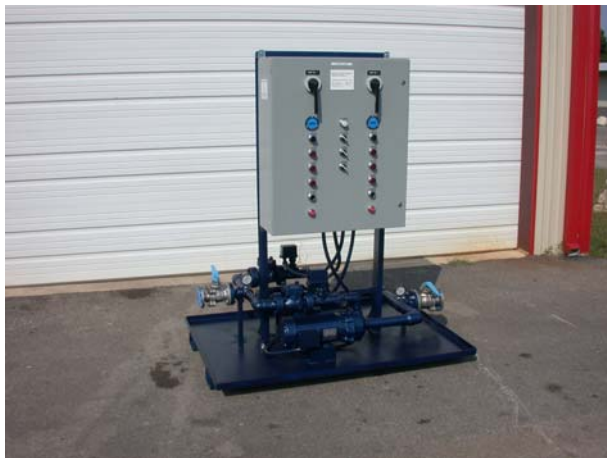
140 GPM De-Min Water Dual Pump System
